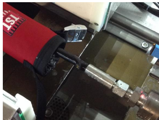
Picture 2: Burst of High Pressure Hose and removed test sample
