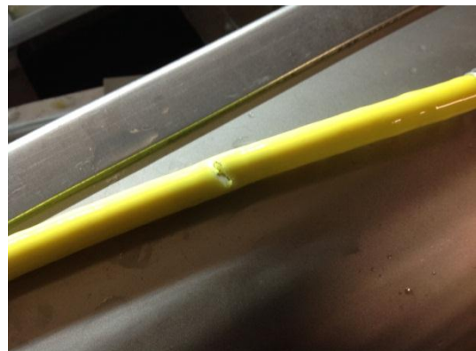
Picture 2: Burst of High Pressure Hose
