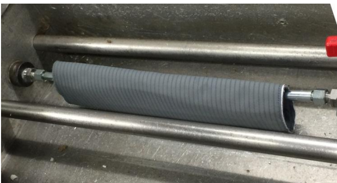
Picture 1: installed High Pressure Hose with Test sample
