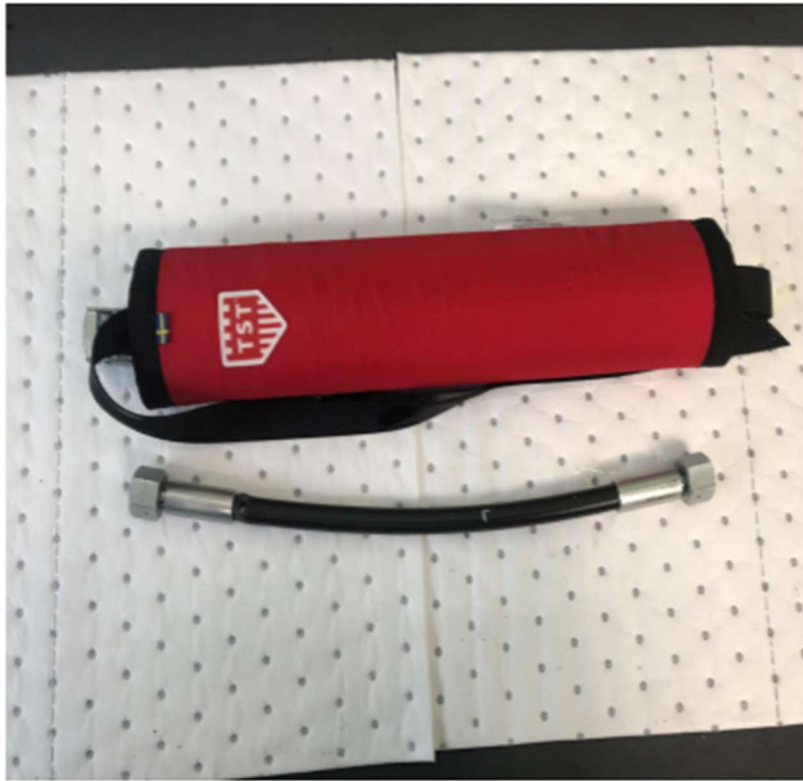
Picture 3: bursted High Pressure Hose with TST hose protection/ shroud, no damage visible.
